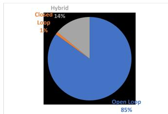
Image 8: Difference in the number of types of ESCG installed on ships.
